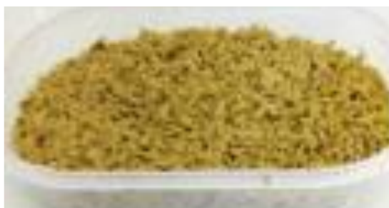
Figure 6: Raffinate obtained by fractionation of cashew apples using a twin-screw extruder
